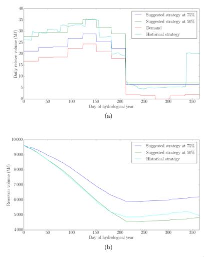
Figure 9: Release strategies suggested by WRDSS at the start of the 2003/2004 hydrological year and corresponding reservoir volume fluctuations for the actual starting volume of the year and a target end volume of  $8000 \text{ M}\ell$ .
