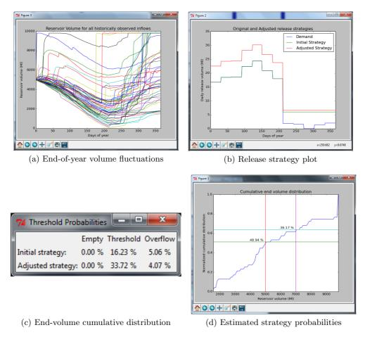
Figure 4: Output produced by the WRDSS concept demonstrator.
