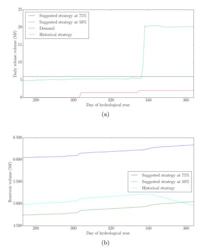
Figure 11: Release strategies suggested by WRDSS nine months into the 2003/2004 hydrological year and corresponding reservoir volume fluctuations for the actual starting volume of the year and a target end volume of  $8\,000$  M $\ell$ .
