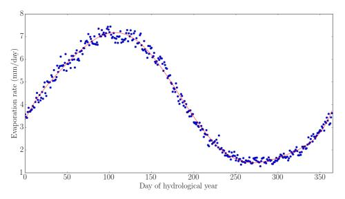
Figure 8: Seventh-degree polynomial fitted to the Keerom Dam daily evaporation rate.
