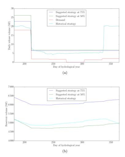
Figure 10: Release strategies suggested by WRDSS six months into the 2003/2004 hydrological year and corresponding reservoir volume fluctuations for the actual starting volume of the year and a target end volume of  $8\,000$  M $\ell$ .
