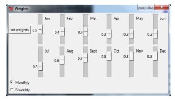
Figure 3: The user interface for specifying the demand-importance weights in the WRDSS concept demonstrator.
