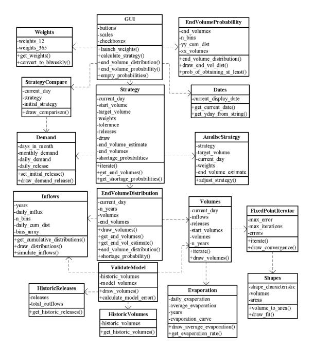
Figure 5: The unified modelling language [22] class structure of the concept demonstrator implementation of WRDSS.
