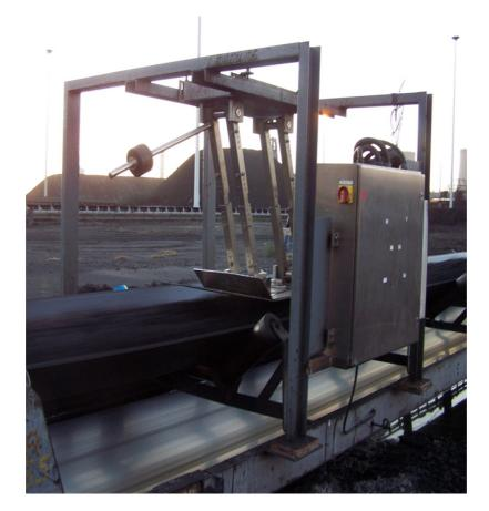
Figure 2: An image of an X-Ray Fluorescence analyser (XRF).
